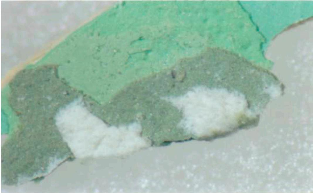
**Fig. 14 Paint Sample WRBR-VC-P032 Removed from a Door in the Office Area of the Wright Brothers National Memorial Visitor Center, Showing Original Green-Colored Paint and White-Colored Primer (Viewed at 30x), (2000).**
