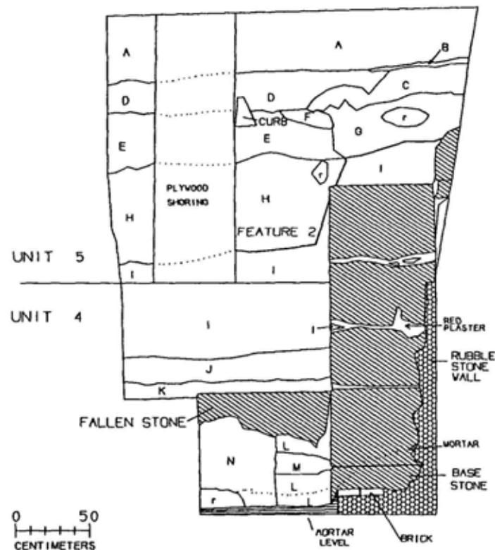
Figure 19. Units 4 and 5, Southeast Profile Showing Unbattered Wall.
