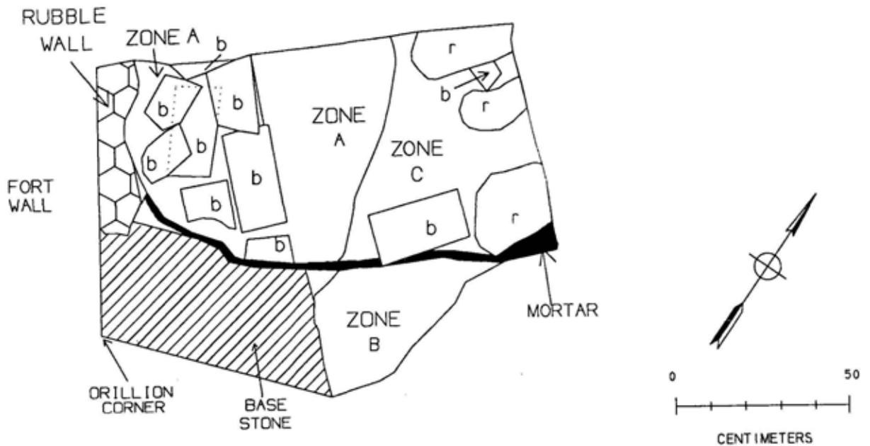
ZONE A: Yellow sand with no aggregate. Possible trench containing large bricks.
