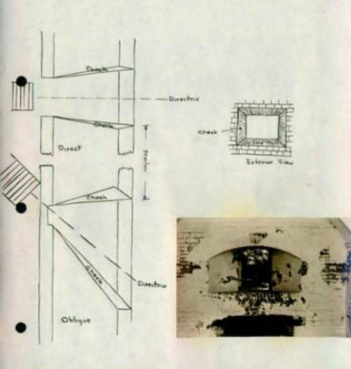
In order that the part of the embrasure which is next to the muzzle of the gun may be nearly of the same width in both the direct and oblique embrasures, the mouth of the latter is wider in proportion to the obliquity. Embrasures are revetted with the same material and in the same manner as the interior slope.
