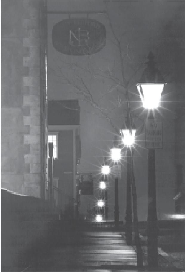
Figure 130: Lantern reproductions, North Water Street. During the 1970s, WHALE's John Bullard had modern incandescent reproductions of nineteenth-century gas lamps cast from two period posts.
