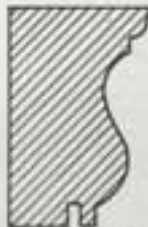
Figure 175. Benaiah Titcomb house, Newburyport, Mass. Detail of excised base of plaster corner with rabbet for clapboards, probably after 1700. (Frame dismantled and re-erected in Faneuil, Mass.)
