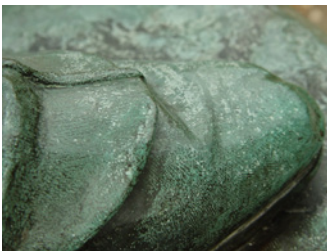
October 2004 Examination of the coating indicated local coating failure (seen as light colored spots) on upper planes of the boots and base.
