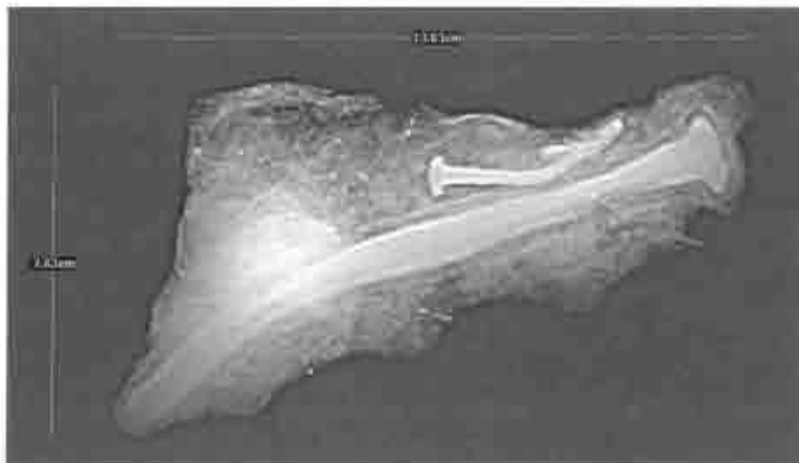
Figure 6.5. Hunhou 99-081A radiograph of concretion showing wrought iron spike and copper-alloy tack. WLCC photo.
