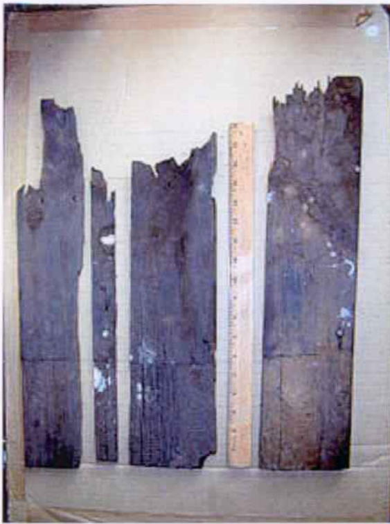
Examples of wood shingles recovered from Henry House attic; shown with 18 inch ruler.
