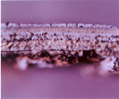
Exterior. Photomicrograph of paint sample MALU A407-413 P14 from an exposed rafter on the south side of the east elevation. Taken at 40X magnification, under reflected tungsten light. Arrow points to the circa-1968 paint layer.
