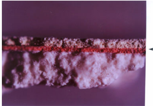
Sanctuary. Photomicrograph of paint sample MALU A407-313 P109 from the circa-1956 south plaster wall. Taken at 40X magnification under reflected tungsten light. Arrow points to the circa-1968 paint layer.
