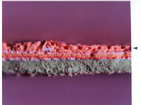
Northwest Stairway. Photomicrograph of paint sample MALU A407-413 P64 from an area of wall surface between the sanctuary and balcony stories covered by the circa-1970 stair. Taken at 40X magnification, under reflected tungsten light. Arrow points to the circa-1968 paint layer.
