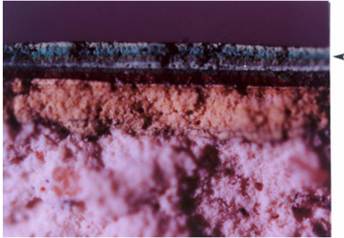
Large Basement Room. Photomicrograph of paint sample MALU A407-413 P18 from the north wall of the large basement room. Taken at 40X magnification, under reflected tungsten light. Arrow points to the circa-1968 paint layer.
