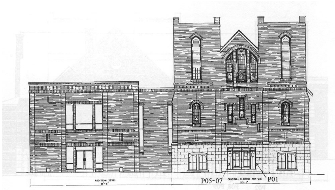
North Elevation. Drawing by the Historic American Buildings Survey, 1985. Annotated with paint-sample locations, May 2000.
