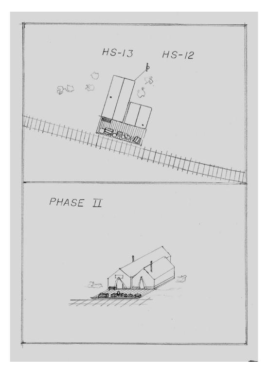
Figure 105. Union Pacific ticket and telegraph office and quarters tents. Note stacks of baggage, boxes and crates as safety block between tents and tracks.
