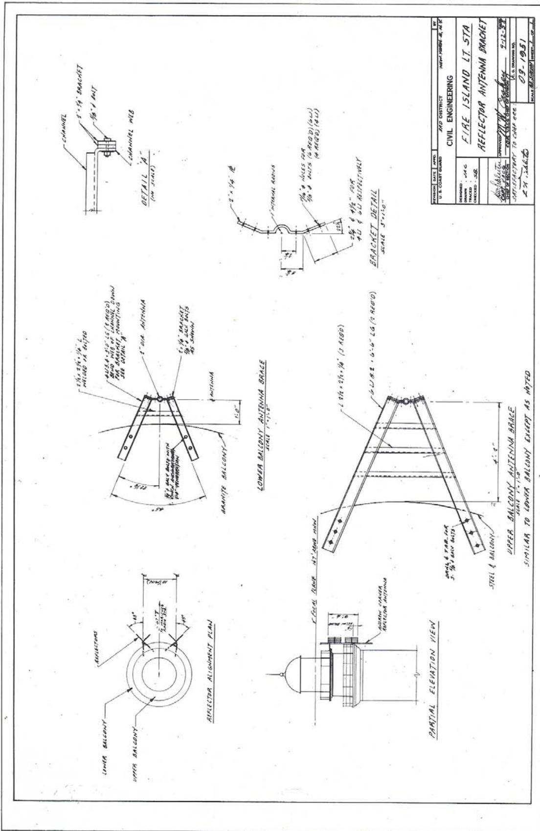
Figure 58. Tower: plan for reflector antenna brackets (1958).
