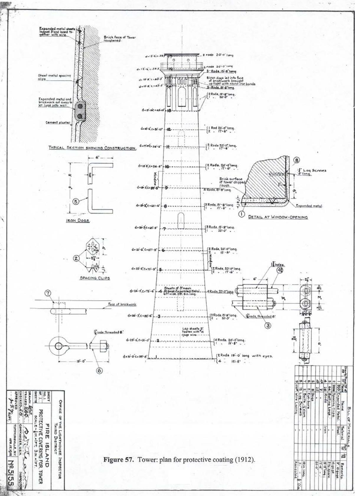
Figure 57. Tower: plan for protective coating (1912).
