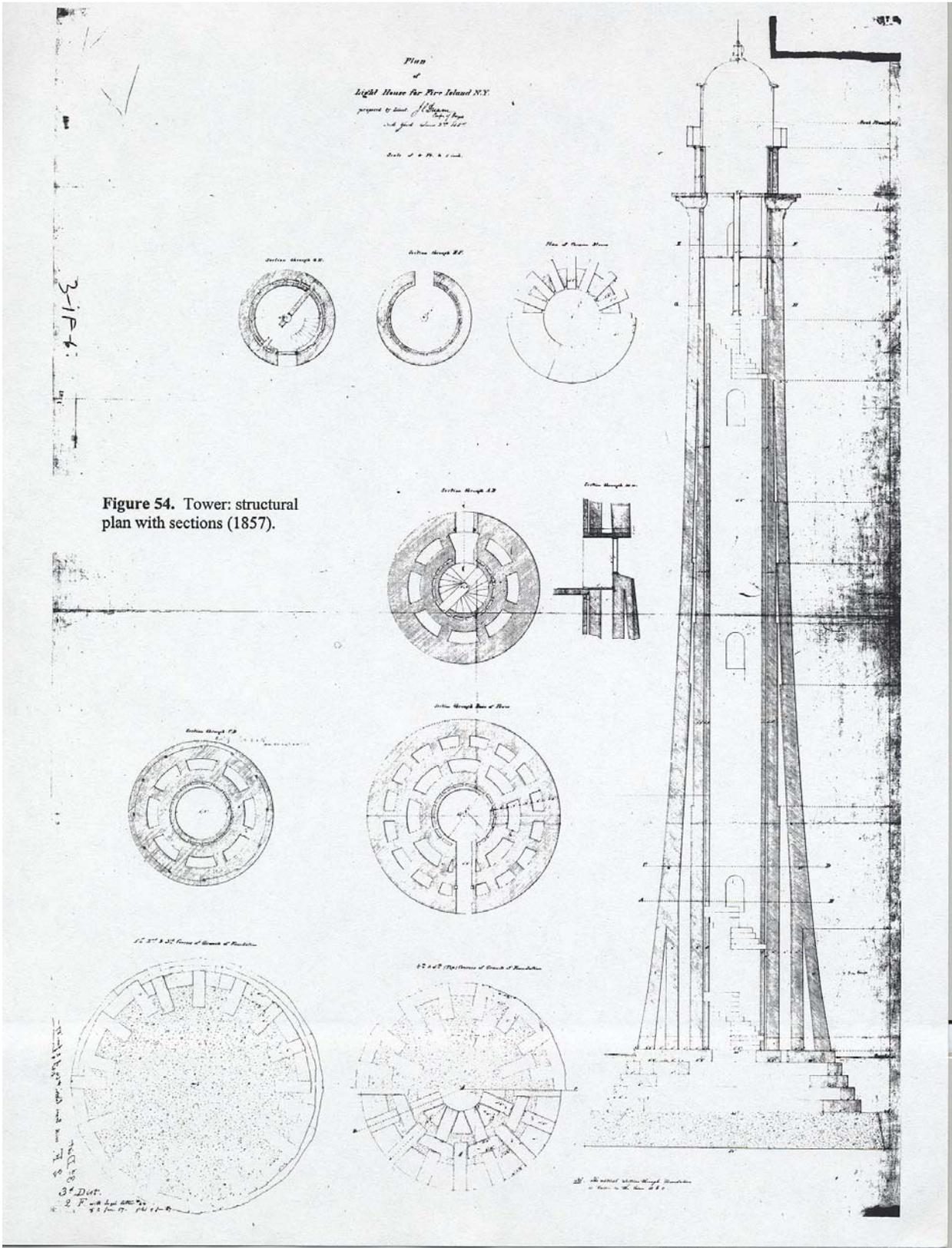
**Figure 54.** Tower: structural plan with sections (1857).
