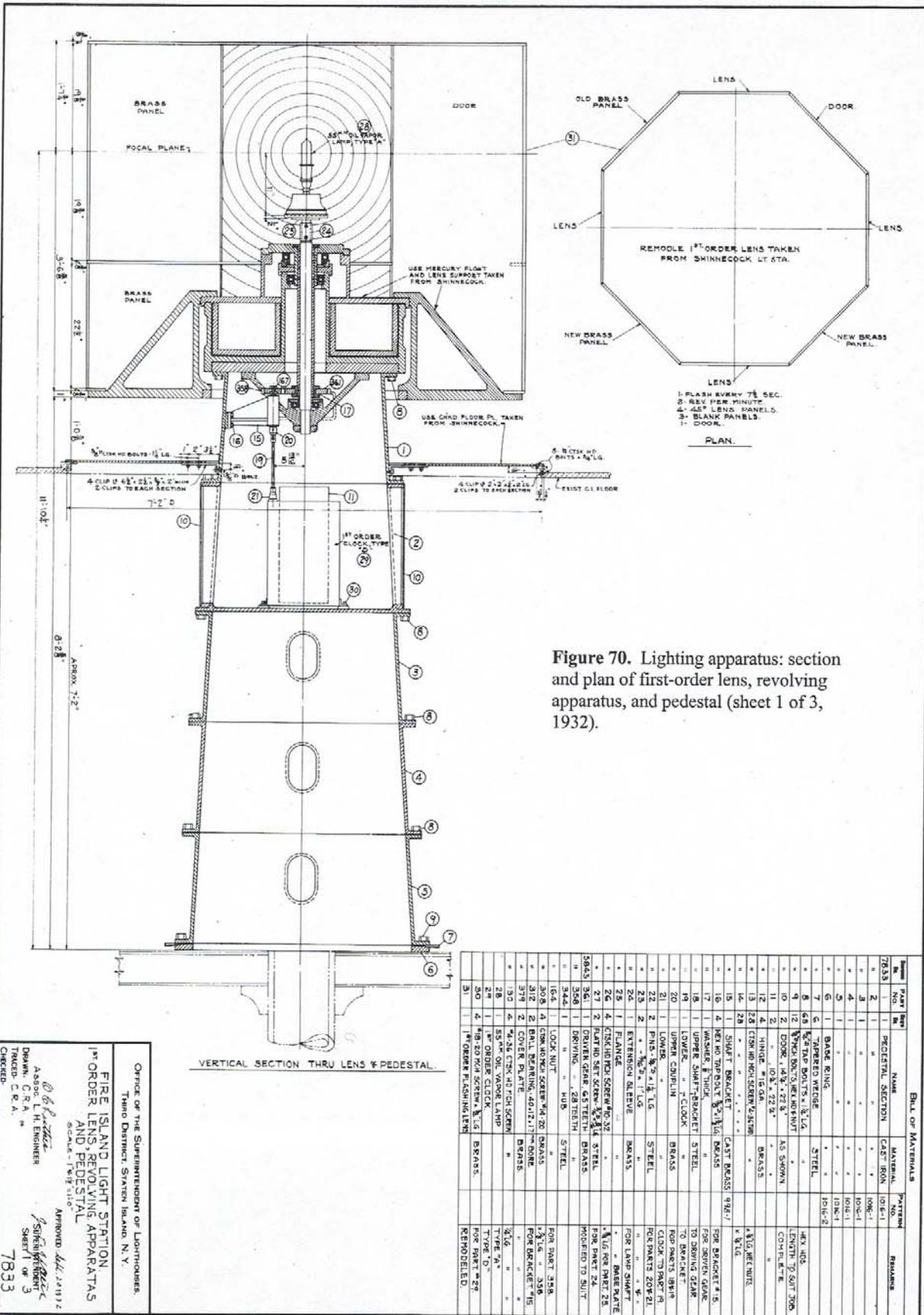
Figure 70. Lighting apparatus: section and plan of first-order lens, revolving apparatus, and pedestal (sheet 1 of 3, 1932).
