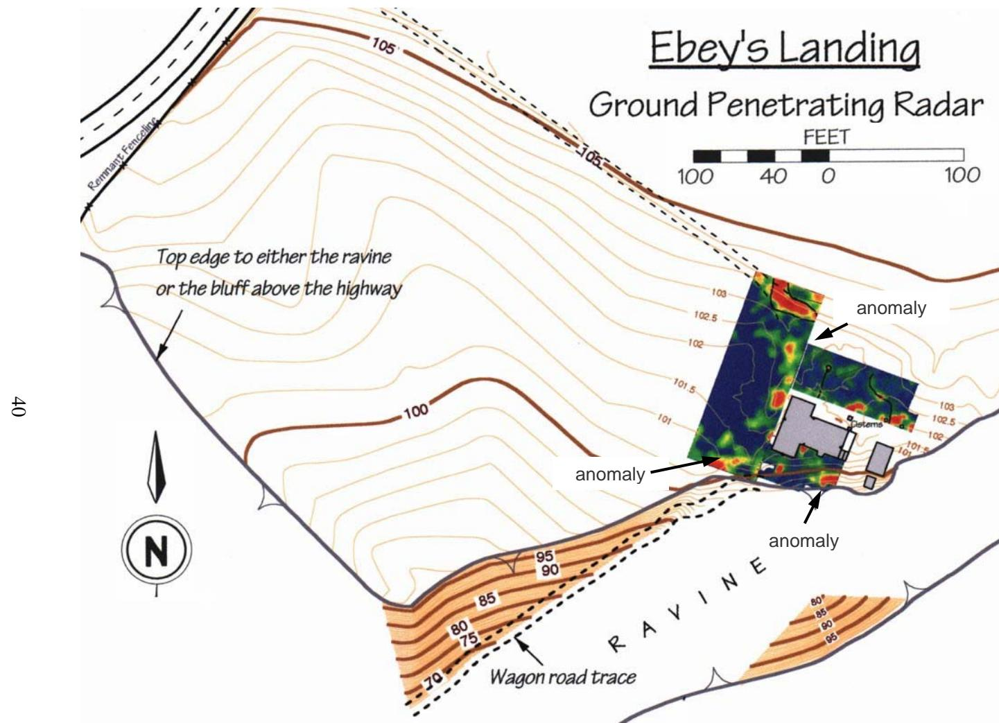
**Figure 12.** Map of ground-penetrating radar survey grid at the Ferry House Site 45IS221. Anomalies are denoted by white outlines. Base map by Keith Garnett, overlay by Larry Conyers.
