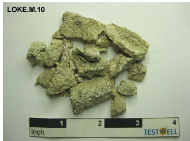
Figure 2: Photographs of mortar samples from the cistern, Kitchen Building and Keeper's Dwelling as received by Testwell for examination.
