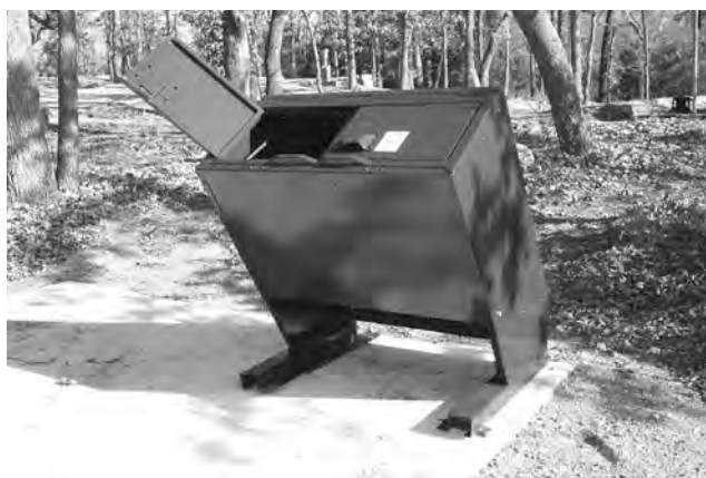
Figure 9-15. Accessible raccoon-proof trash receptacle, used elsewhere in the CNRA. The doors on this model open horizontally instead of vertically.
