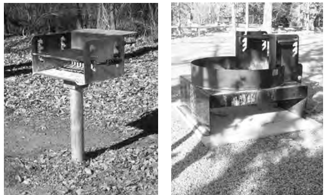
Figure 9-12. Pedestal grill (left) and fire ring grill (right) currently used in the park. The fire ring, on a concrete pad, has an ADA-accessible, adjustable grill.
