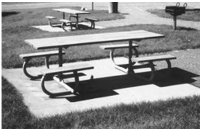
Figure 9-34. A typical, fully accessible picnic area requires hardened access and surface.
