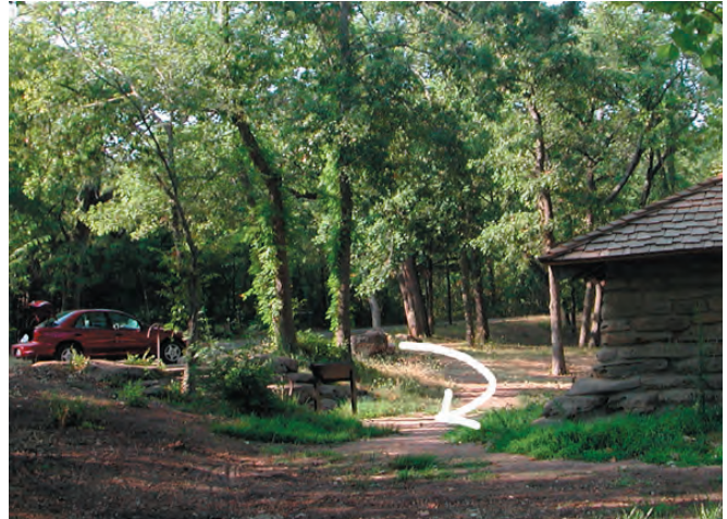
Figure 11-67. Improved, if not full, ADA access can be provided by constructing a ramp between the parking area and the entrance to the pavilion, along the arrow shown in the photograph.
