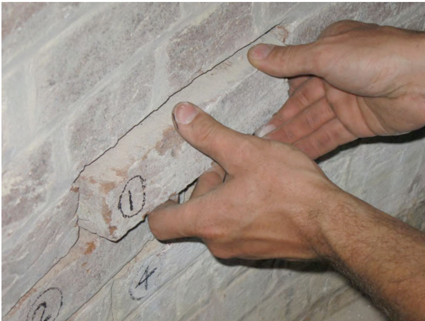
Figure 4. Cape Lookout Lighthouse, October 2008. Removal of a brick for laboratory testing. A total of five bricks were removed from the building. Photograph by author.
