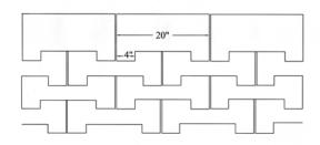
**Figure 10** Pattern of midtwentieth century asphalt shingles on Styron House. (NPS-SERO-CRS, 2001)
