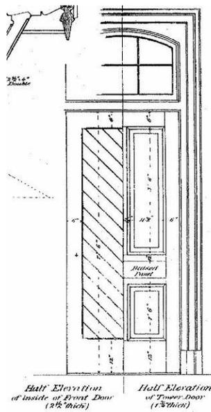
**Figure 17** Original drawing of front door details.
