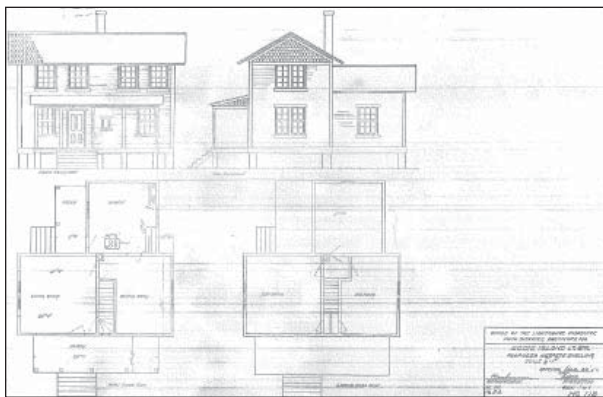
Figure 9, Plans for proposed Principal Keeper's dwelling at Bodie Island Light Station, December 30, 1906. (CAHA collection)
