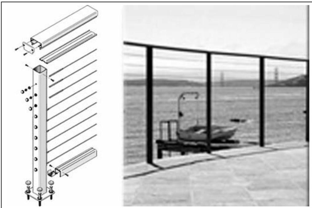
**Examples of tension cable fencing. Left: schematic drawing; Right: unobstructed views of a harbor through a fence (Feeney Gateway, [http://www.cablerail.com/index\\_2.html](http://www.cablerail.com/index_2.html)).**
