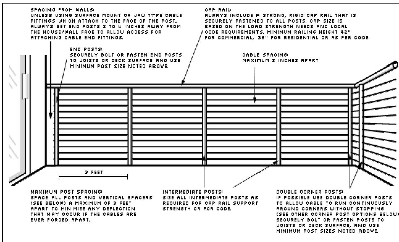
Example of a tension cable fence with double corner posts and no foot rail (Feeney Gateway, [http://www.cablerail.com/index\\_2.html](http://www.cablerail.com/index_2.html)).
