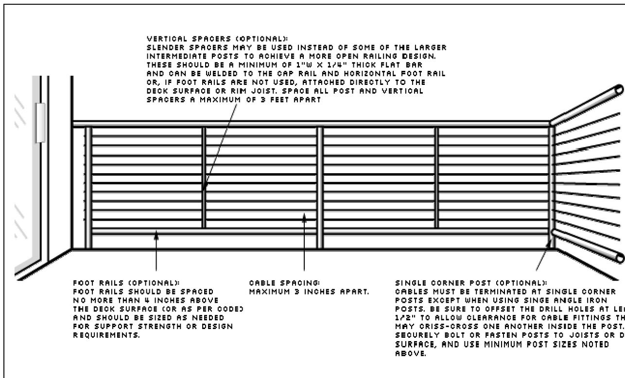
Example of a tension cable fence with a single corner post and a foot rail (Feeney Gateway, [http://www.cablerail.com/index\\_2.html](http://www.cablerail.com/index_2.html)).
