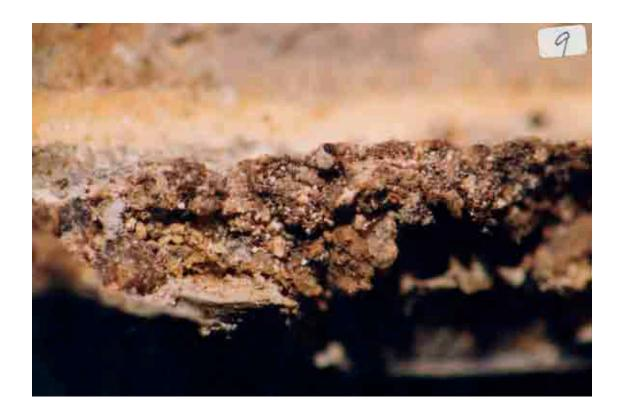
Figure 4. Photomicrograph of brown coating suggests possible sanded paint, to replicate brownstone, perhaps. The thickness, texture, and inharmonious color may be reasons why it was mostly removed.
