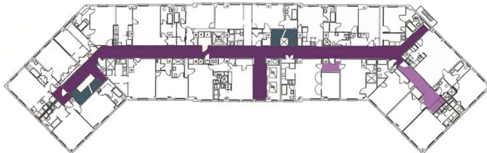
Post-rehabilitation plan of typical upper floor. Corridors and staircases have survived intact. Former fire escape “accessways” have been absorbed into two apartments and a vestibule is absorbed into one apartment on each floor. Shown in lavender are intact, previously public areas (a small vestibule and the end leg of the corridor) that have been incorporated into two of the apartments on each floor.
