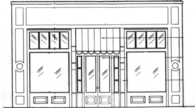
Inappropriate entrance design.
