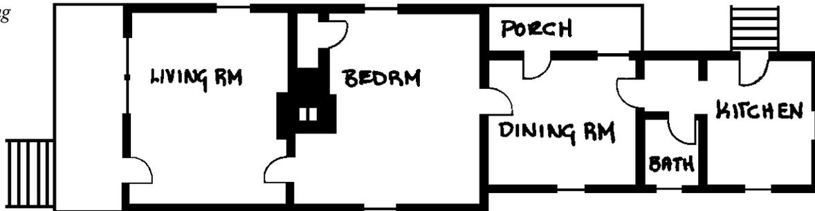
Plan: Before. Note the typical historic linear plan of this shotgun house and the need to move through rooms from front to back. This open plan works well with one bedroom, but does not afford adequate privacy when two bedrooms are needed. Note also the small open side porch which is subsequently enclosed.
