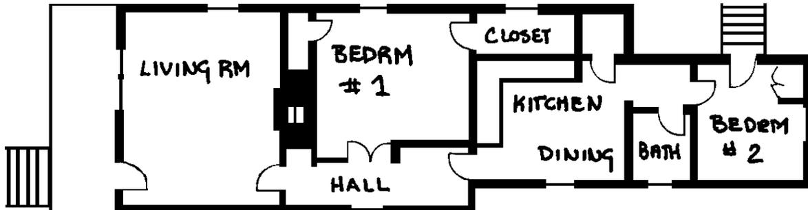
Plan: After. Note the placement of the former kitchen into the dining room which allows the rear room to be changed into a small bedroom. The added wall at the middle of the building creates a small corridor to give privacy to the master bedroom. Most trim, the windows, and fireplace surrounds were retained.
