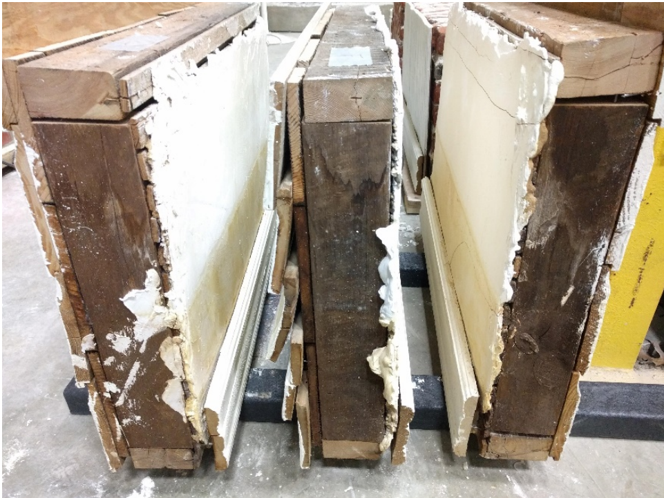
Figure 42. Photograph of Wall C, D, and F frames showing wicking of the treatment solution and subsequent mold growth during the drying phase.
