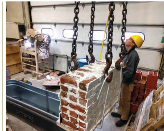
Fig. 3. Wall assemblies that were too heavy for two people to lift into and out of the immersion tank were hoisted by a crane. The wall assemblies were constructed on small wood platforms, and steel bars were used to create hooks with which to lift the samples. Courtesy of ERDC/CERL TR-19-8, 2019.
