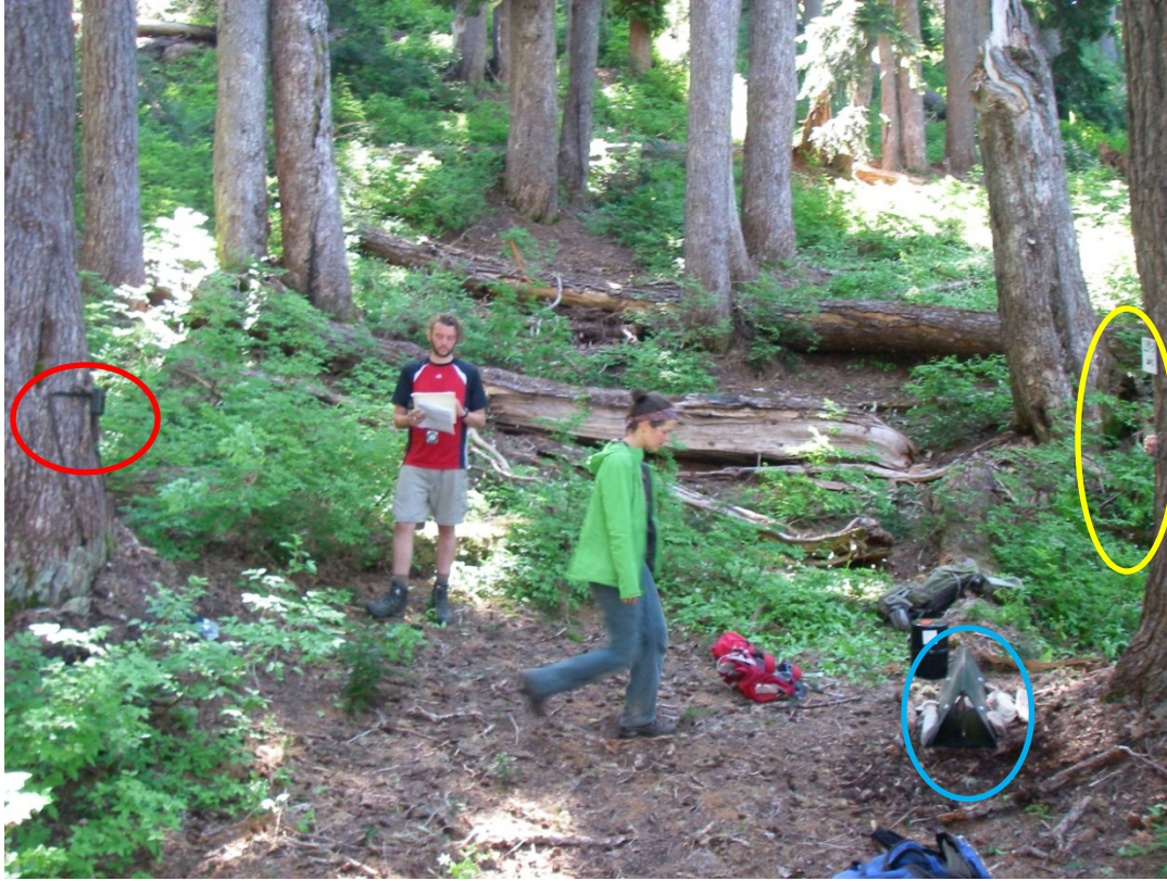
Figure 3. Members of a field crew setting up a station within Olympic National Park (Hex 239). Note camera (circled in red) on left of frame is pointing to tree bait (yellow circle) and baited cubby (blue circle) box on the right of the frame.
