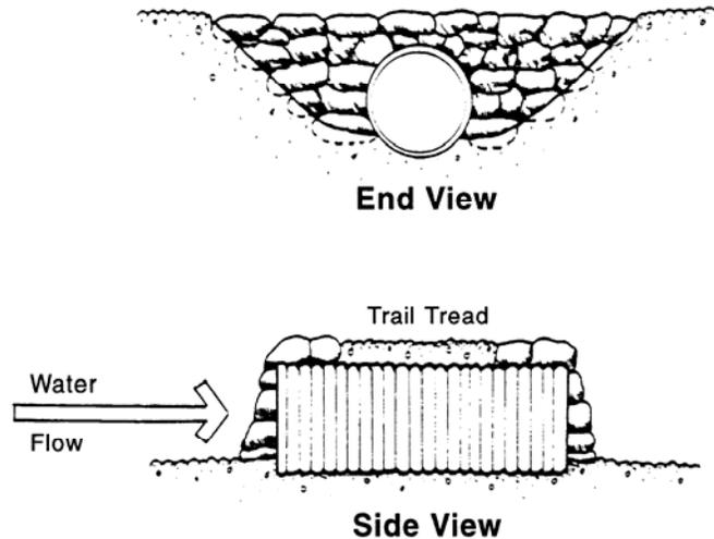
Culverts may be more cost effective and less obtrusive than a bridge. They are easier to install in most instances.
