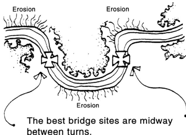
Whenever possible, the entire wet area should be spanned, or ramps used to get onto an elevated bridge. This eliminates the need for steps which are an accessibility barrier. As seen in the section on steps and perrons (later in this chapter) it is recommended that steps be minimized.
