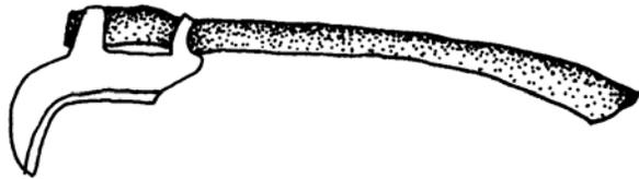
**Tips:** The blade should be kept sharp using a curved-edge whetstone.
