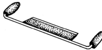
**Tips:** Users should acquire a true draw knife that has its handles at a right angle to the blade—rather than a bark knife that has handles in line with the blade. Bark knives are meant only for smoothing rough bark—not removing it.
