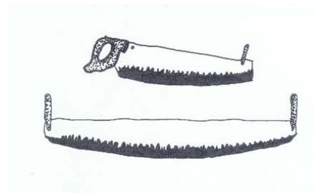
only alternative for cutting large material. In less remote areas, they are used only occasionally as the axe, bowsaw, and chainsaw perform the same jobs.
