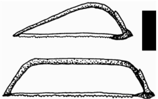
**Tips:** Bow saws cannot be resharpened due to the hardness of the blade. When the blade becomes dull, rusty, or bent, it should be replaced. It should be wiped with light oil before storing. Smaller saws are more useful—use another tool for cutting large material.
