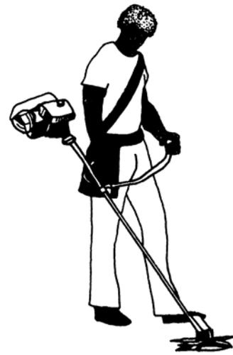
**Tips:** Brushsaws come in a variety of sizes. Trail work requires a more powerful unit than one that is used for lawn trimming. Generally, a brushsaw with an engine of 35cc to 80cc and bicycle-type handlebars is recommended. For durability, a known brand such as Stihl, Husquevarna, or Jonserud should be obtained. These saws also come with a variety of blades depending on the material to be cut. Trail work requires a saw type or a universal grass-brush blade—not a string cutter.
