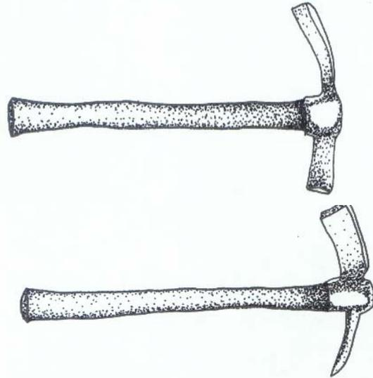
There are two kinds of mattocks—pick mattocks and cutter mattocks. Both have an adze blade, but the pick mattock has a pick, opposing the adze, whereas the cutter mattock has a cutting blade. The pick mattock is most useful in hard or rocky soil where the pick is useful to break up the soil or pry out rocks. The cutter mattock is more useful in deeper, rooty soil where the cutter is needed to sever roots.
