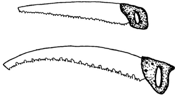
**Tips:** Pruning saws should be resharpened often. A light coat of oil should be applied to the blade after each use.
