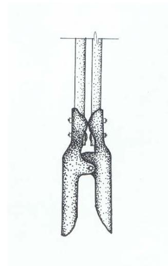
**Safety:** Soil should be lifted from the hole with leg muscles—not back muscles. If the wooden handles are too flexible or the collar becomes bent, fingers can get pinched when the handles are closed. Leather gloves are recommended.
