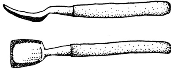
**Tips:** The spud has three cutting edges. All three should be sharpened on the top side only. A file should be used—a fine edge is unnecessary. Timbers peel much easier during the spring when the sap is flowing freely. Logs can be peeled in the spring and stockpiled for later use during the construction season.
