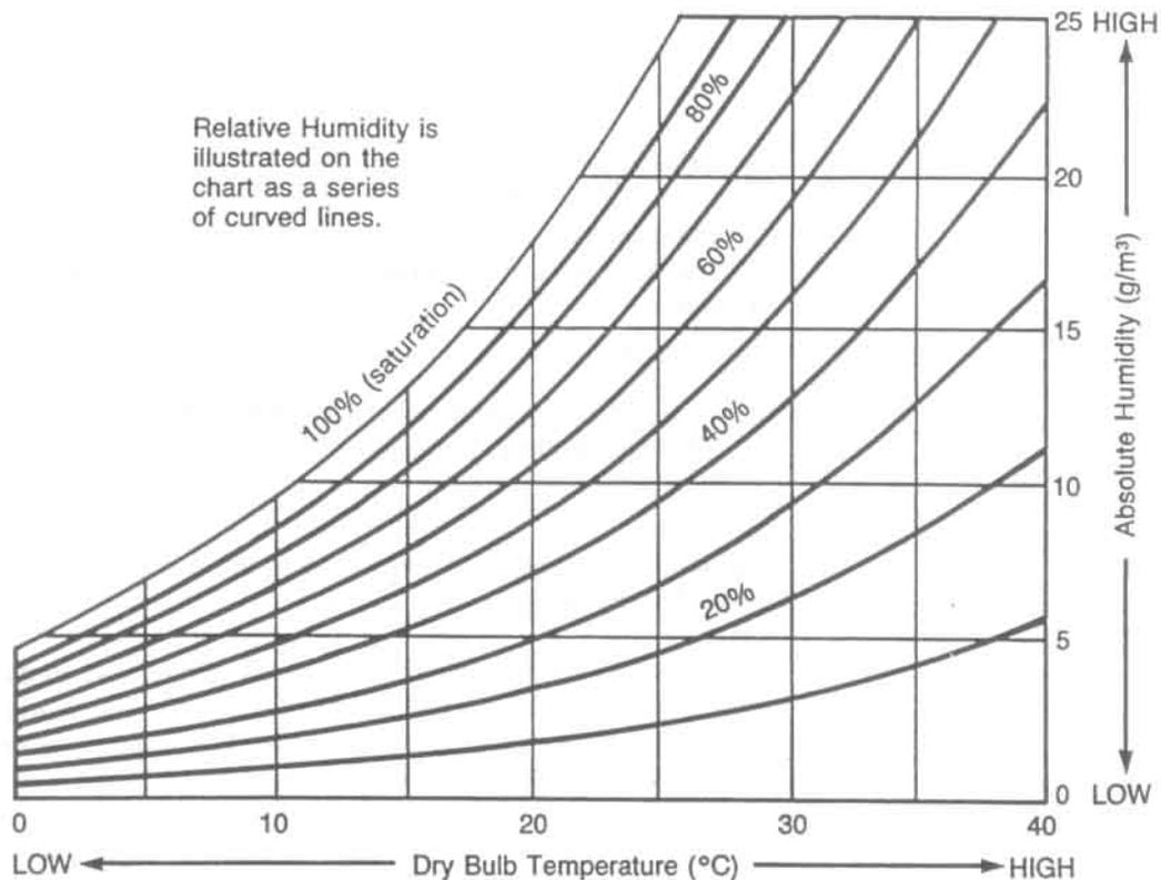
Follow any horizontal line (representing a specific amount of moisture in the air) from left to right on the chart (i.e., from lower to higher temperature levels). Note that RH decreases as temperature increases, so long as the quantity of moisture in the air does not change.
