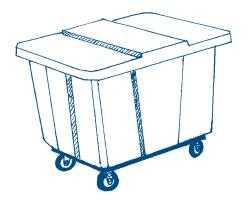
Figure 1. Rigid polyethylene bin on wheels
