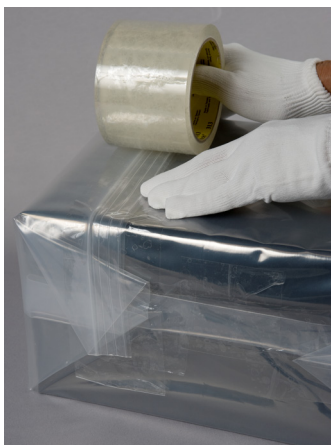
Figure 6. The sealed “zipper-lock” end of the outer bag is taped flat to the box.
