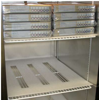
Figure 2. Ethafoam™ sheets used to line wire shelves.
