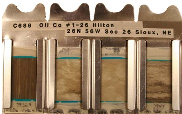
Figure 2. Geological thin sections made from a drill core.
