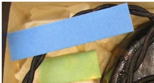
Figure 1. Blue A-D test reference strip above reacted green/yellow A-D strip
