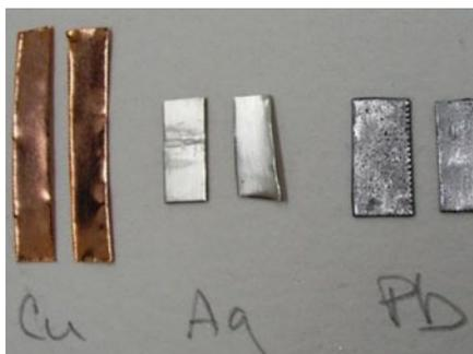
Figure 2. Copper (Cu), Silver (Ag) and Lead (Pb) coupons cut and cleaned for monitoring.
