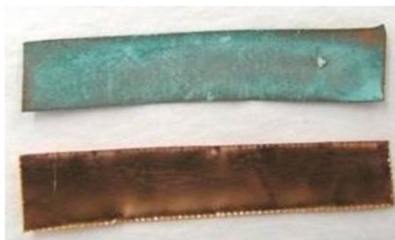
Figure 3. Top: Copper coupon after 4 weeks of exposure to off-gassing cellulose nitrate
