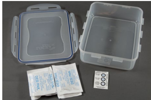
Figure 2. Microclimate box components; box, desiccant, and humidity indicator.
