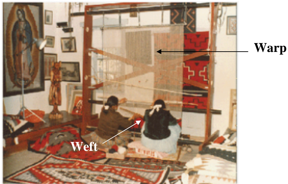
Figure K.1. Upright loom. (Weavers Mae and Sadie Curtis of Ganado at Hubbel Trading Post. Photograph by Fred Mang Jr. HUTR-23347)
