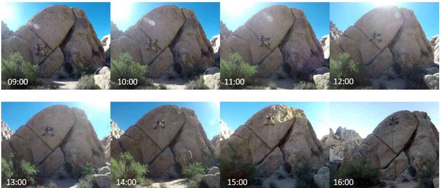
Figure 5. A sequence of photographs of LEMUR showing climbing progress at Sweeney Granite Mountains Desert Research Center. LEMUR climbed approximately 4.2 meters in seven hours.
