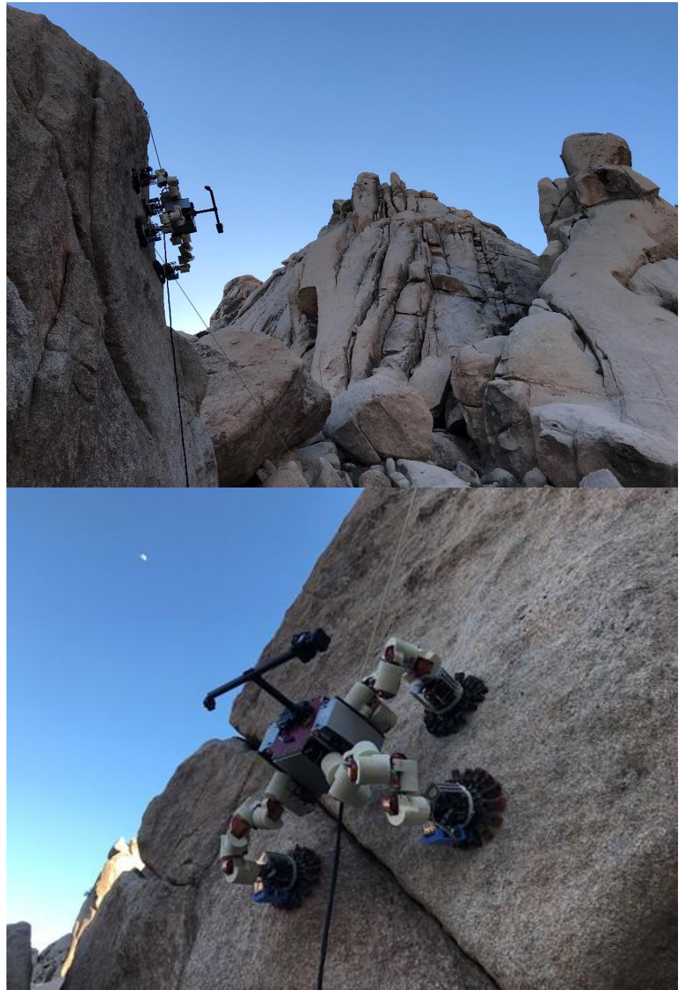
Figure 1. LEMUR scaling a nearly vertical granite outcrop at the Sweeney Granite Mountains Desert Research Center. Microspine gripper end effectors are attached to the chassis via seven degree-of-freedom limbs. A perception system consists of a camera and LIDAR mounted to a mast on the chassis. A safety line and a tethered power cable are also present above and below LEMUR.
