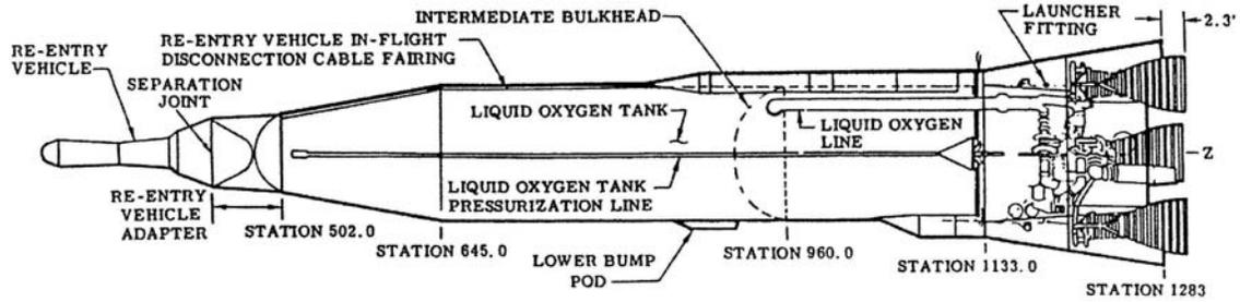
Plate 6. Cutaway drawing of an Atlas D ICBM. Later Atlas E and F missiles used the same airframe but added more powerful engines (*John C. Lonquest and David F. Winkler, To Defend and Deter: The Legacy of the United States Cold War Missile Program* (Washington, D.C.: Department of Defense, Legacy Resource Management Program, 1996), 210)
