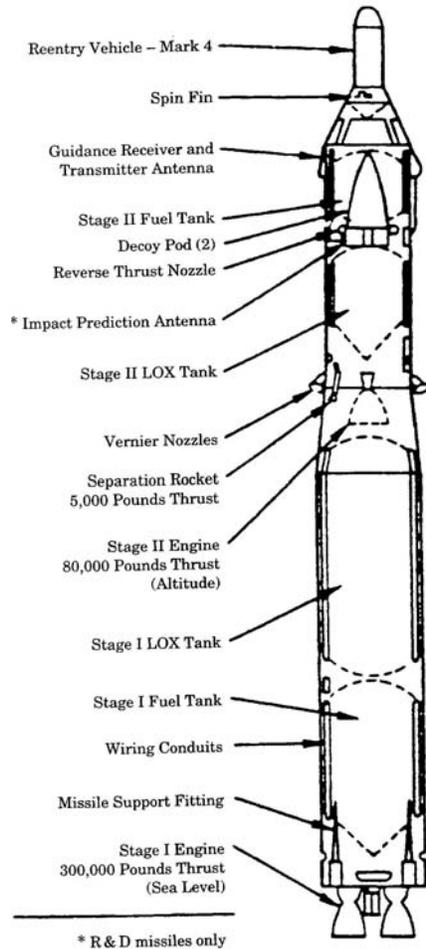
Plate 7. Drawing of Titan I, the United States' first two-stage ICBM (*Lonquest and Winkler, To Defend and Deter: The Legacy of the United States Cold War Missile Program*, 228)
