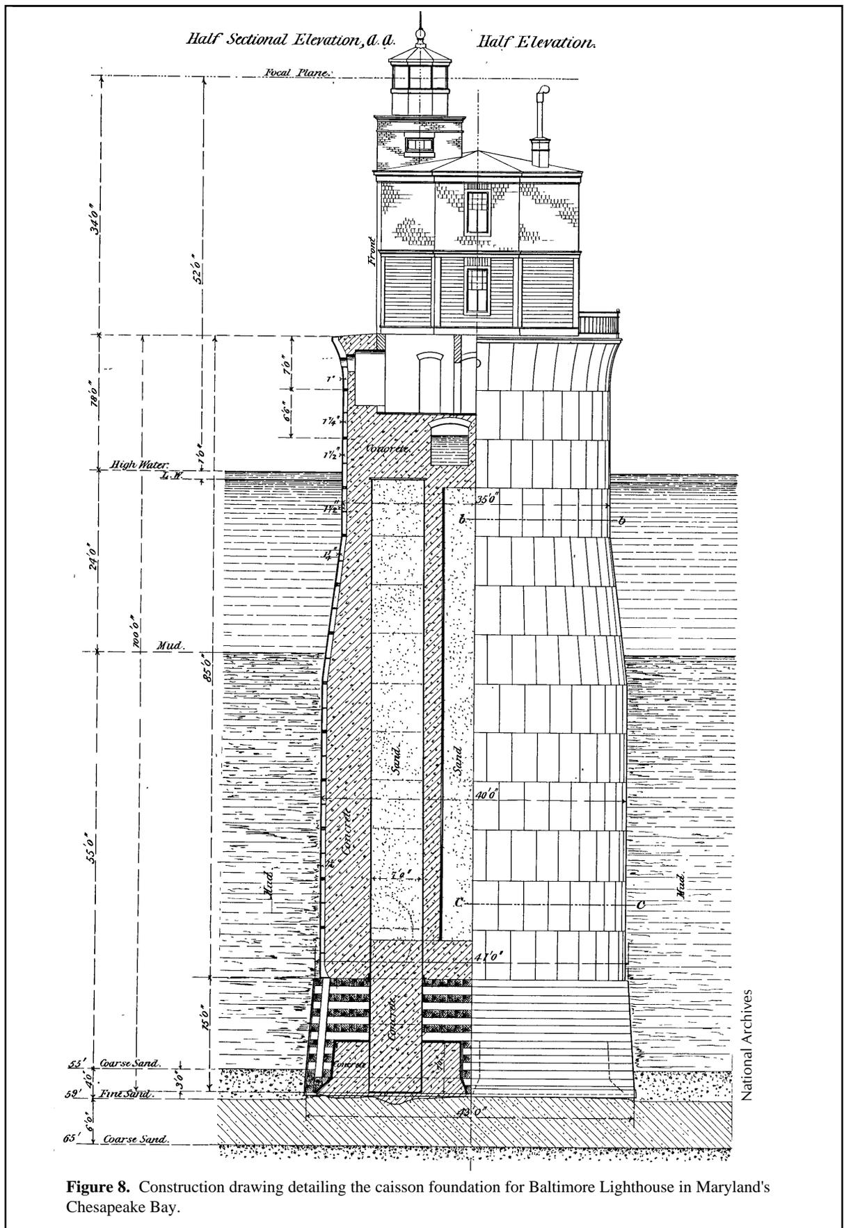
**Figure 8.** Construction drawing detailing the caisson foundation for Baltimore Lighthouse in Maryland's Chesapeake Bay.
