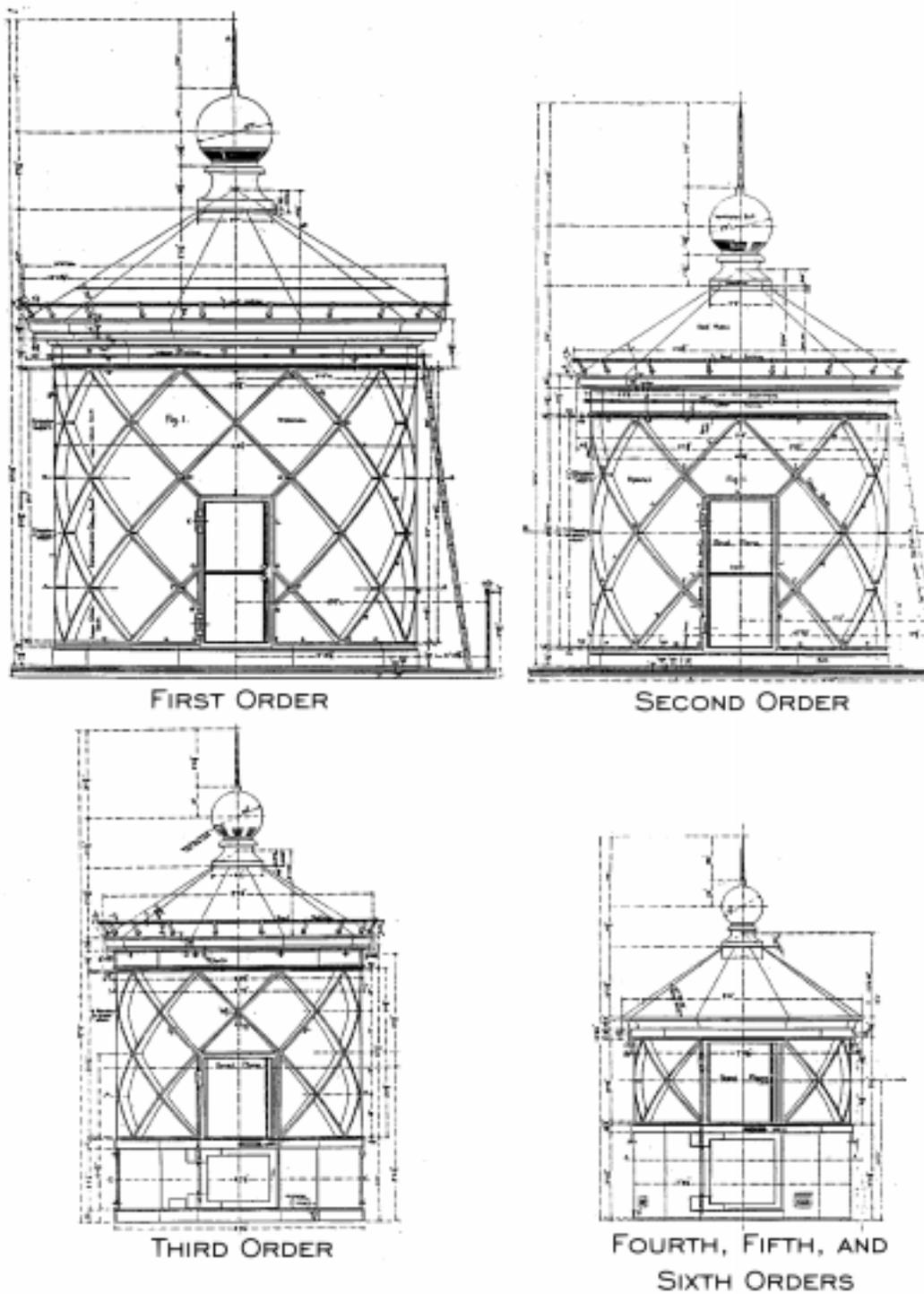
**Figure 3.** Illustration of the four standard lantern sizes used by the U.S. Lighthouse Establishment in the first half of the 20th century. Drawing assembled by WPTC from images dated 1898 and 1903 courtesy of USCG CEU Oakland.
