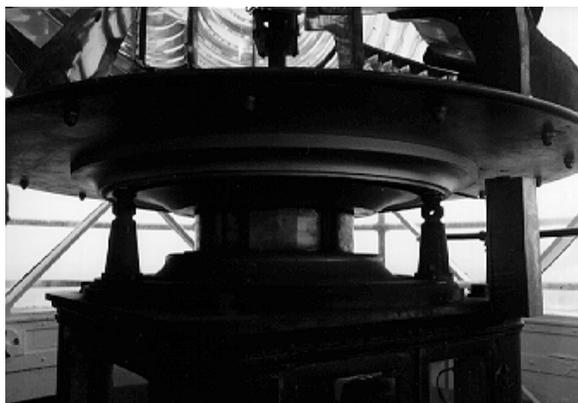
**Figure 36.** This c. 1926 lens was designed to be AC powered; the original lens jacks are still in place. The three jacks (the third is obscured by the brass bearing cover) were used to lift the lens assembly so that bearings could be serviced.
