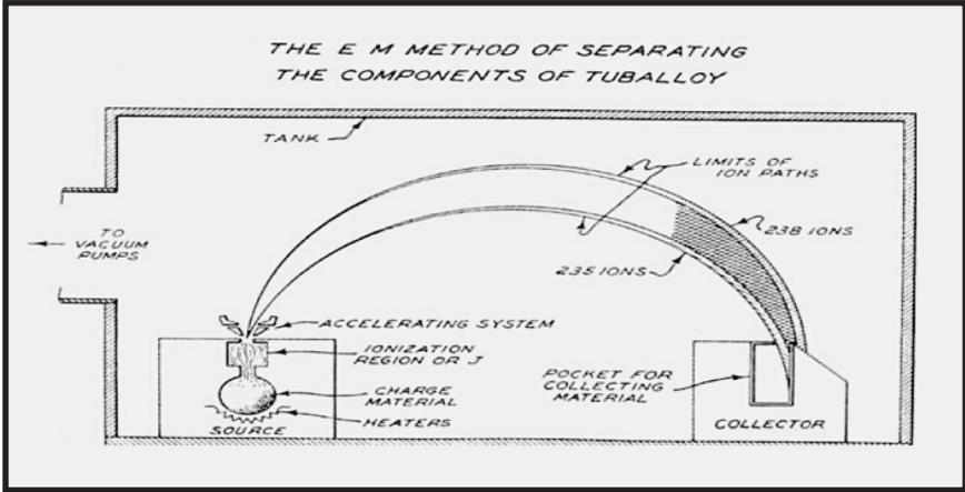
Diagram of uranium isotope separation in the calutron.
