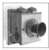
Late in Alice Longfellow's lifetime, she had a second call bell system installed. Made by the American Telephone & Telegraph (Bell) Company, this early telephone intercom system can be seen on the kitchen's south wall and on a wall in Alice Longfellow's second-floor bedroom. It let Alice speak directly to the cook and other staff in the kitchen.
