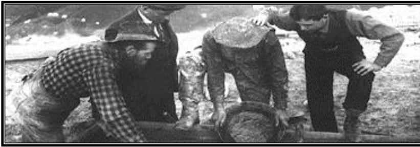
pieces of gold are picked out by hand or with tweezers. Finer grained gold is separated from the commonly associated black sand by using a magnet. After drying, a magnet will attract the magnetite, or "black sand," and leave the gold. "Flour" gold will typically be removed from the remaining sediment by mercury amalgamation. Mercury is placed in the pan, where it readily forms a mixture, or amalgam, with the gold. The amalgam is then heated. The mercury vaporizes and the gold remains.
