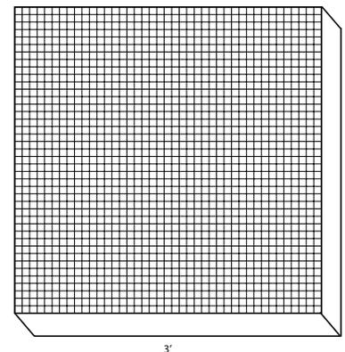
Nail four 2" x 4" x 3' boards together to form a 3' x 3' (1 meter) square. Staple gun fine mesh to the bottom.
