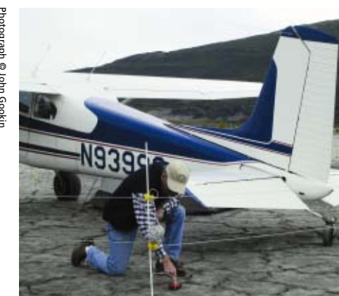
Electric fencing is an option to protect aircraft at remote landing sites.
