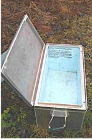
Heavy gauge aluminum is an excellent material for bear-resistant boxes and panniers. Boxes should meet USFS criteria for bear-proof containers, which include: "(a) resist a direct force of 200-pounds; and (b) contain no cracks, external hinges, gaps, etc. by which a bear can force the container open using claws or teeth."
