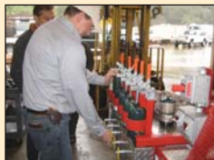
Yosemite National Park uses a propane bottle recycler to recover leftover propane so that the empty bottles can be recycled with other metals.
