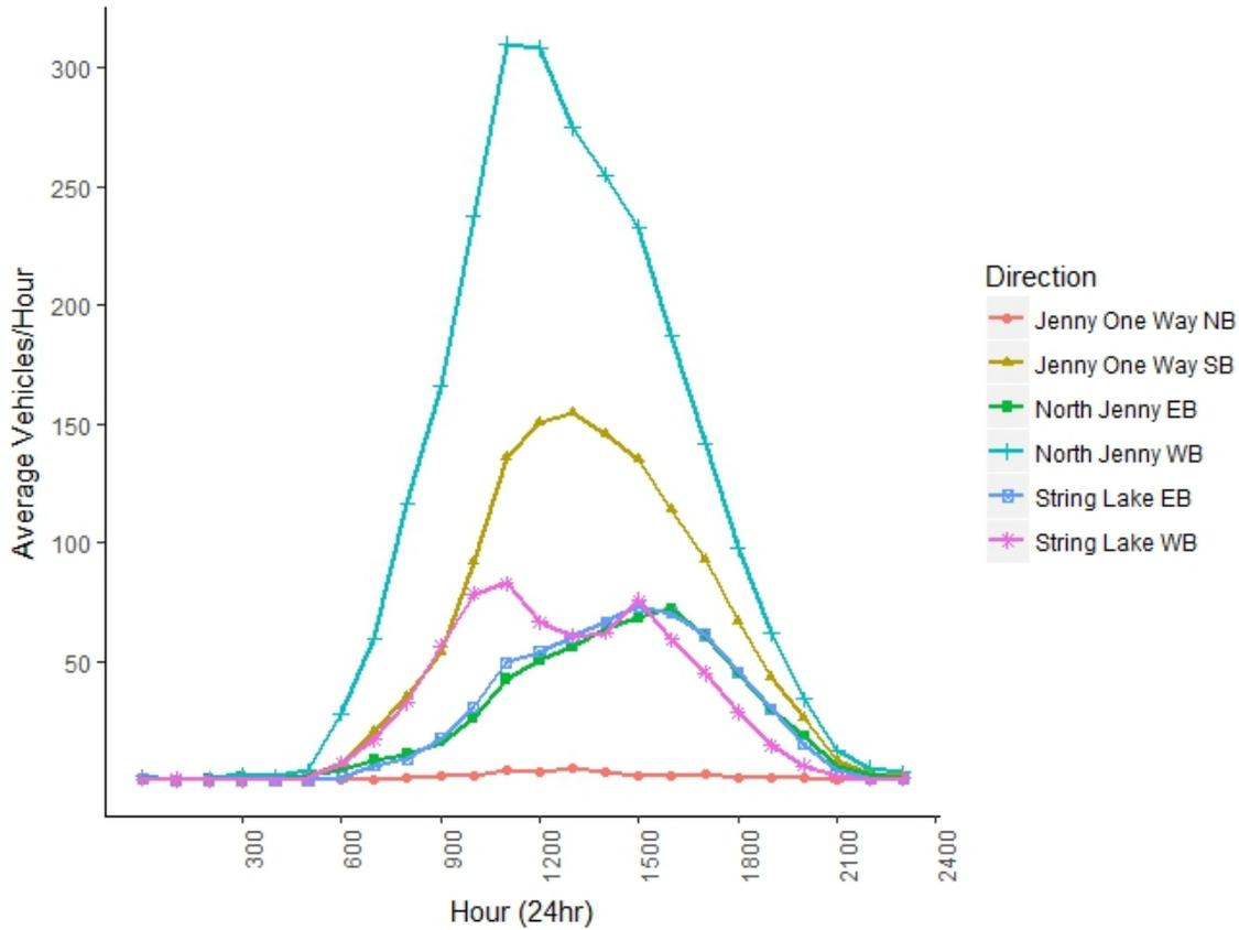
**Figure 8a.** Average hourly directional counts for all three MetroCounters placed in the String Lake study area during the summer sampling period (July 15 – August 15) on **weekdays**. NB = northbound, SB = southbound, EB = eastbound, WB = westbound. String Lake WB are vehicles driving towards the North Lot, String Lake EB are vehicles driving towards the exit. Jenny Lake One Way tube malfunction resulted in no data from August 9 to August 17.
