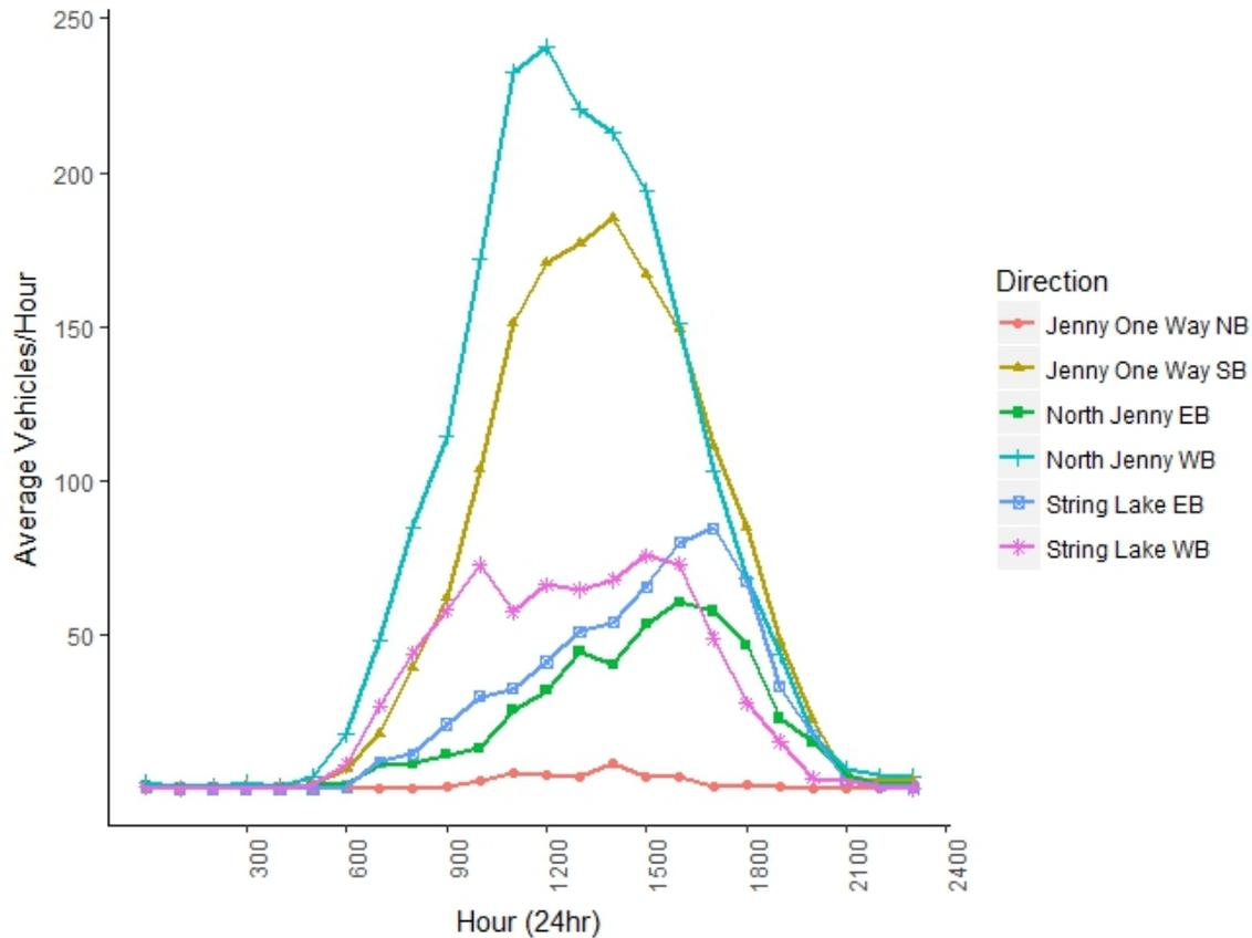
**Figure 8d.** Average hourly directional counts for all three MetroCounters placed in the String Lake study areas during the shoulder sampling period (August 16 – September 8) on weekends. NB = northbound, SB = southbound, EB = eastbound, WB = westbound. String Lake WB are vehicles driving towards the North Lot, String Lake EB are vehicles driving towards the exit. Jenny Lake One Way tube malfunction resulted in no data from August 9 to August 17.
