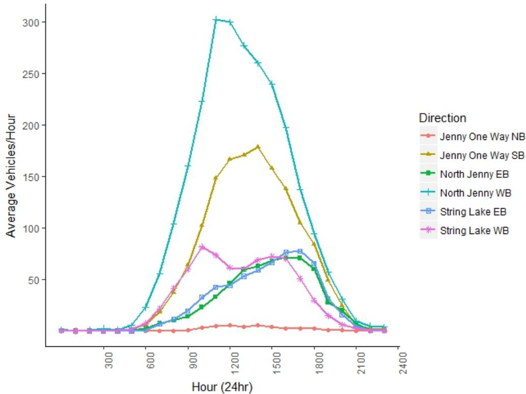
**Figure 8f.** Average hourly directional counts for all three MetroCounters placed in the String Lake study areas across both sampling periods (July 15 – September 8) on **weekends**. NB = northbound, SB = southbound, EB = eastbound, WB = westbound. String Lake WB are vehicles driving towards the North Lot, String Lake EB are vehicles driving towards the exit. Jenny Lake One Way tube malfunction resulted in no data from August 9 to August 17.
