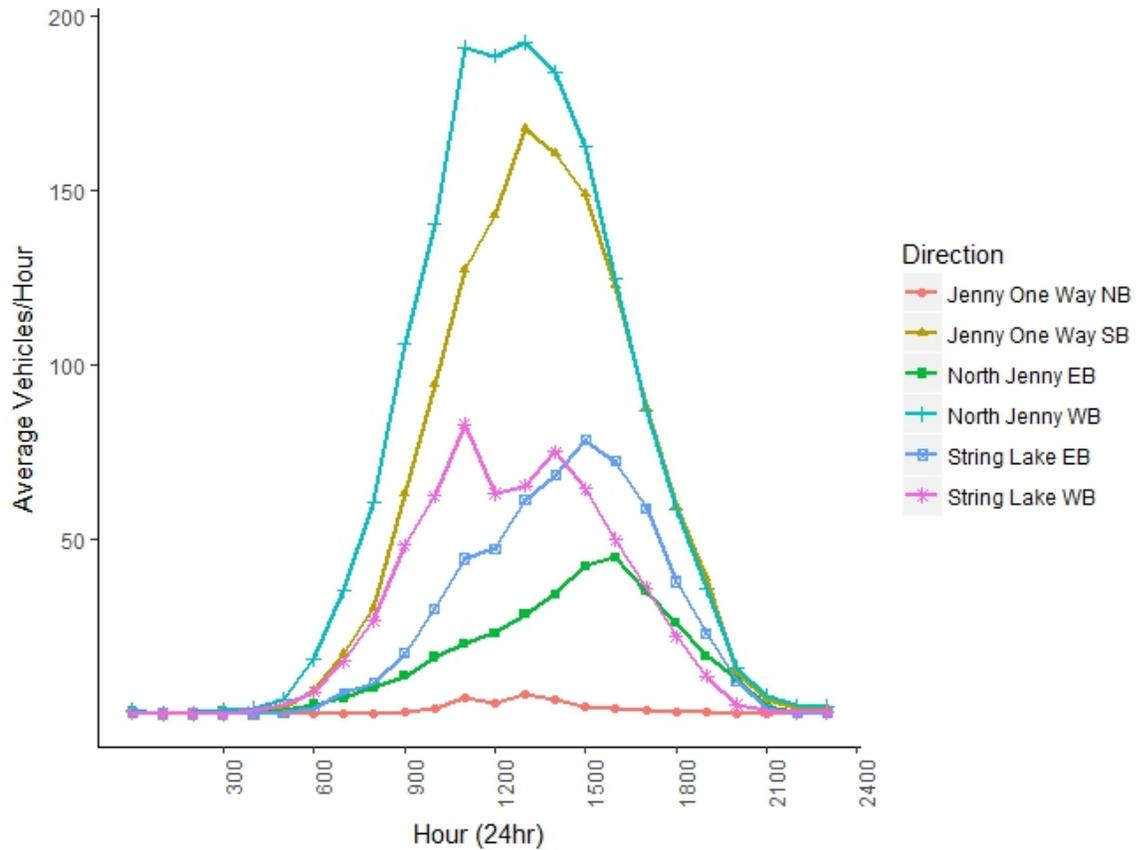
**Figure 8c.** Average hourly directional counts for all three MetroCounters placed in the String Lake study areas during the shoulder sampling period (August 16 – September 8) on **weekdays**. NB = northbound, SB = southbound, EB = eastbound, WB = westbound. String Lake WB are vehicles driving towards the North Lot, String Lake EB are vehicles driving towards the exit. Jenny Lake One Way tube malfunction resulted in no data from August 9 to August 17.
