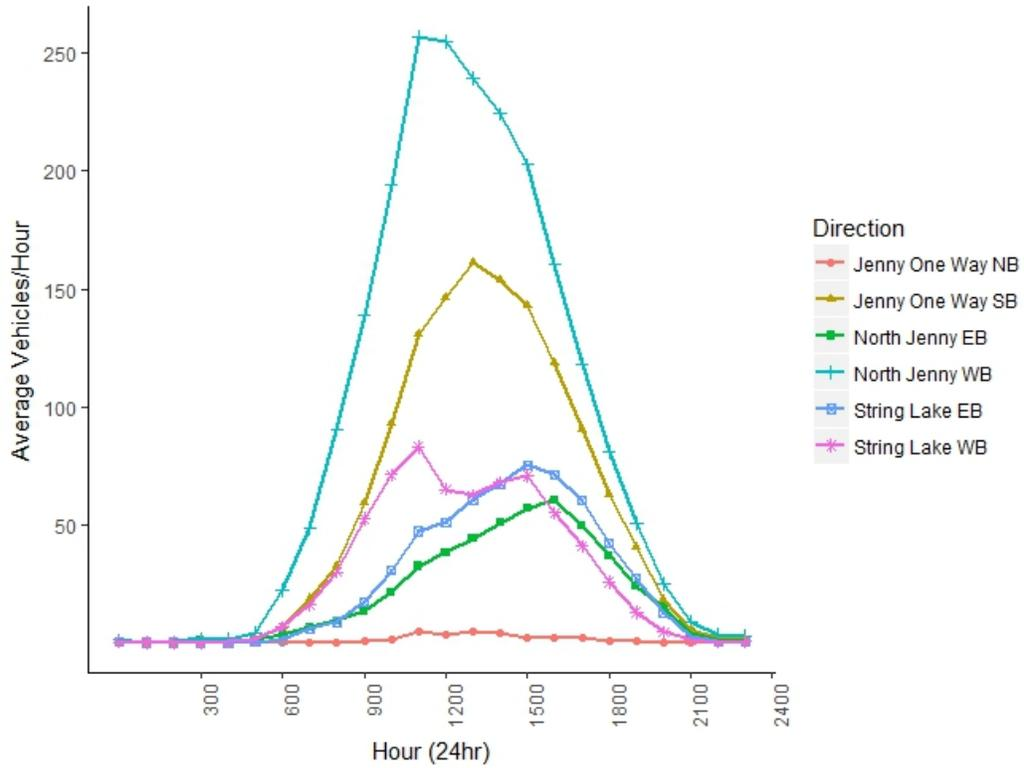
**Figure 8e.** Average hourly directional counts for all three MetroCounters placed in the String Lake study areas across both sampling periods (July 15 – September 8) on **weekdays**. NB = northbound, SB = southbound, EB = eastbound, WB = westbound. String Lake WB are vehicles driving towards the North Lot, String Lake EB are vehicles driving towards the exit. Jenny Lake One Way tube malfunction resulted in no data from August 9 to August 17.
