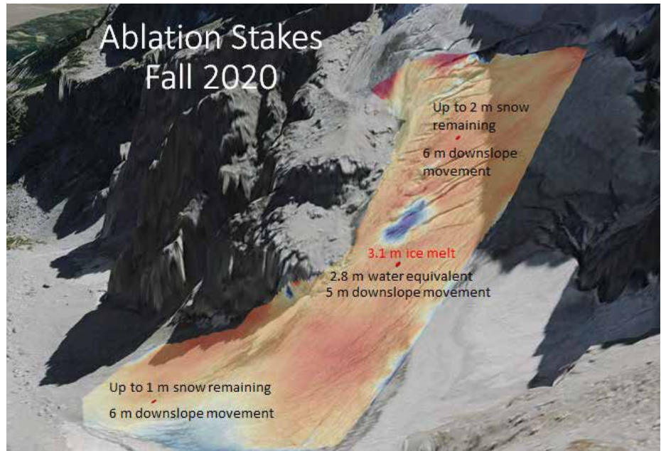
Ablation stake results from fall 2020: Oblique view of Middle Teton Glacier with 3 of 5 ablation stakes locations depicted with the amount of ice melt or snow remaining and glacier velocity.
