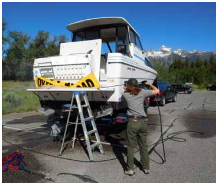
An AIS inspector uses a hot-water sprayer tool to decontaminate a boat that was last on Lake Powell, a quagga mussel infested lake.
