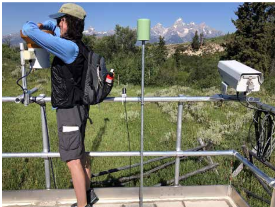
Park staff maintain the air quality station which includes a webcam that shows current visibility.
