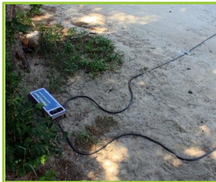
Figure 1.1: Tube counter used to determine vehicle use levels on the Death Canyon Road (photo by Ashley D’Antonio).
