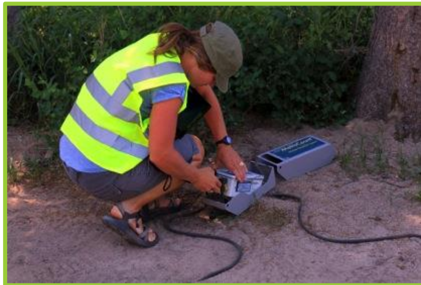
Figure 4: Field technician, Annie Weiler, downloading data from the tube counter on Death Canyon Road during Summer 2013. The same tube counters were used during Summer/Fall 2014 (photo by Ashley D’Antonio).
